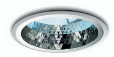
Compatta-Faceted Body and reflector in polycarbonate (UL94VO) self-extinguishing, under vacuum metallized reflector. IP44 screen included.
