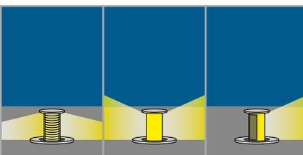
The Movi light source can be free or diffused using additional anti glare plates. It is also possible to limit distribution to 180° with blanking screen.
