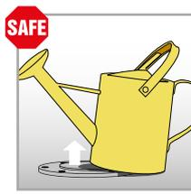
When a weight is placed on top of the Movi, restricting its upward movement, the fitted safety sensor restricts the movement of the fitting. When weight is removed it will operate normally.
