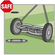
With the correct mounting of Movi in a grassed area when recessed, grass can be cut easily without any obstacles.
