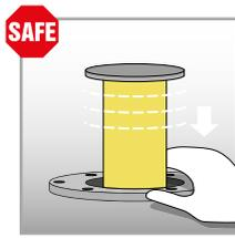
Should an object impede closure of Movi as it is retracting, the protective metallic cover will detach ensuring the main body of the fitting still descends inside its housing. Once obstacle is removed, the metal cover can easily be re-attached.
