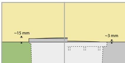
By using the additional plastic ring, you have the possibility to mount Movi to ground level.
