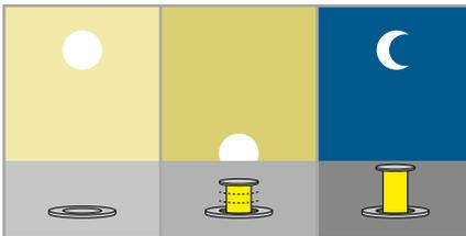
Wiring option: if Movi is connected to a photocell or time clock, the switching can be automated.
