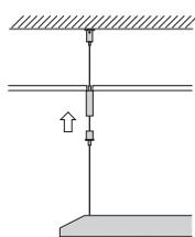
The kit makes it possible to mount the suspension cables directly on the ceiling, without losing the possibility of adjusting the length, for cases in which there is a false ceiling that might not be able to withstand the weight of the luminaires.
