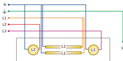
With Extrudo, a single fixture can provide the right amount of lighting at all times. In fact, it is possible to obtain individual switching of the different light bulbs present in a single luminaire by using more than one power line.
