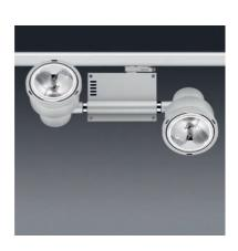
Track light with two heads for HIR111 lamps. Housing made of die-cast aluminium, powder-coated in matt grey metallic. Rotatable and adjustable. HIR 111 version c/w electronic ballast. Beam angle acc. to lamp. Incl. universal adapter for 3-phases track. Max. weight: 2.1 kg
