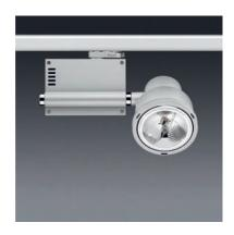
Track light for HIR111 or HIT-CE lamp. Housing made of die-cast aluminium, powder-coated in matt grey metallic. Rotatable and adjustable. C/w electronic ballast. HIT-CE reflector made of matt pure aluminium, beam angle 2 x 30°. HIR111 beam angle acc. to lamp. Incl. universal adapter for 3-phases track. Max. weight:  $1.4 \, \text{kg}$
